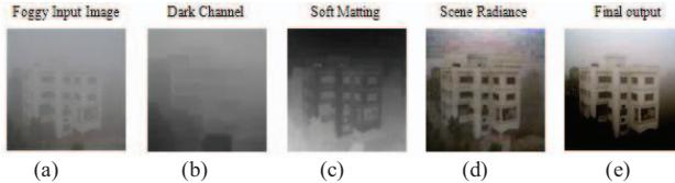
Fig. 2. (a) Real time fog degraded input image (b) Corresponding image using Dark Channel Prior (c) Corresponding image using Soft Matting (d) Corresponding image using Scene Radiance (e) Final output image.[7].
