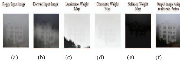
Fig. 1. (a) Foggy input image (b) Corresponding derived input image (c) Corresponding Luminance Map of enhanced image (d) Corresponding Chromatic Map of enhanced image (e) Corresponding Saliency Weight Map of enhanced image (f) Fog-free output image by performing multiscale fusion [10].
