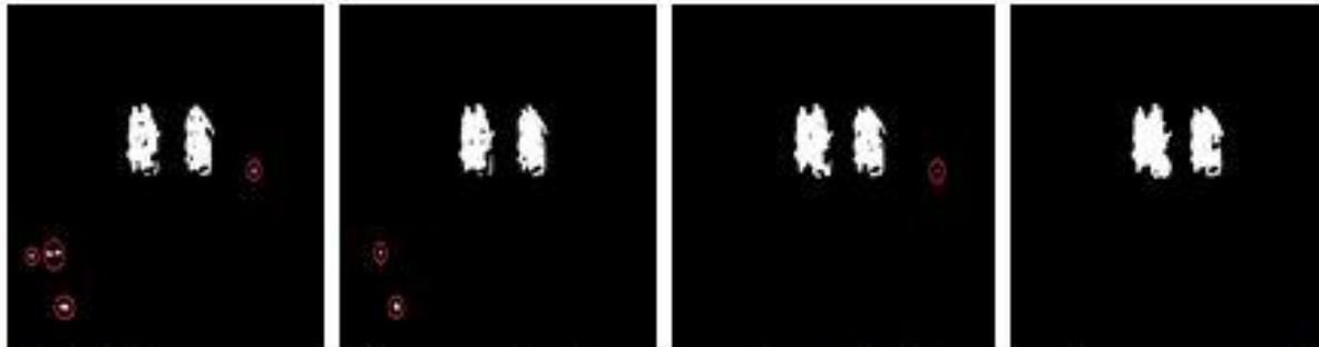
Fig. 8. Sequence of segmented frames, where the incorrectly segmented (marked by red circles) foreground pixels are gradually vanish in subsequent frames.
