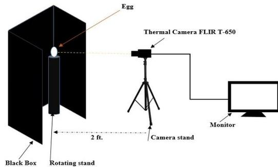
Fig. 2. Diagrammatic Representation of Overall Acquisition Setup
