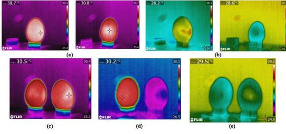
**Fig. 3 Sample Images of Created Dataset (a) Fresh Eggs; (b) Defective Eggs; (c) Two Fresh Eggs; (d) One Fresh and One Defective Egg; (e) Two Defective Eggs**
