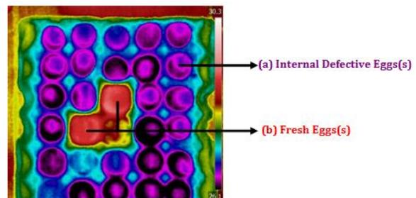
Fig. 1. Infrared Imaging (Top View) of Bunch of Eggs Kept in Trays: (a) Internal Defective Eggs; (b) Fresh Eggs
