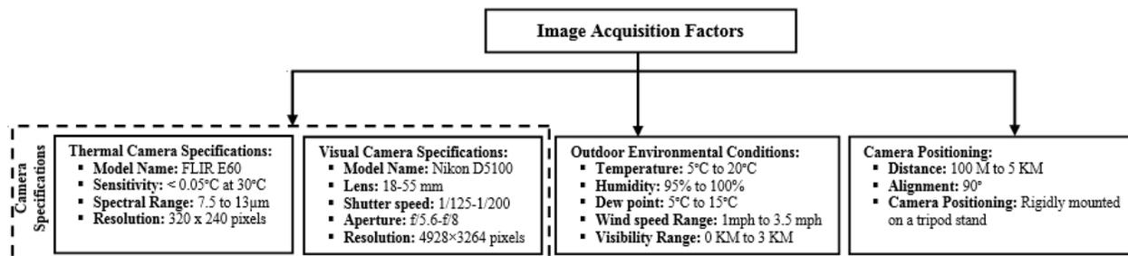
Fig. 1 Camera Setup and Acquisition Factors for Capturing Natural Scene Images of SAMEER-TU Database
