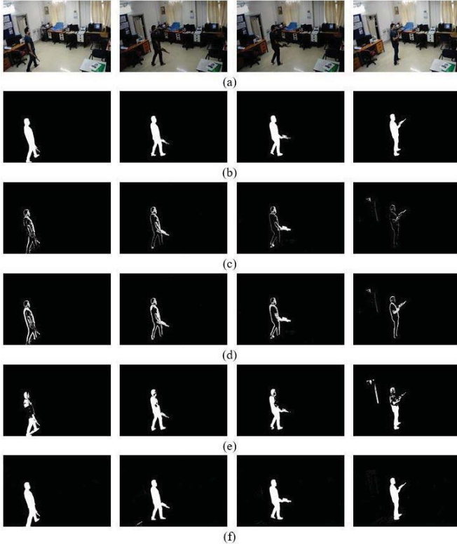
Fig. 5. (a) Original Video frames and (b) ground truths. The remaining four sub-pictures present the binary mask of moving objects generated by the (c) GMM [9], (d) MTD [10], (e) ViBE [11], (f), and ISBS [12] approaches.
