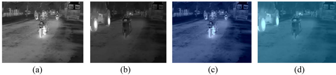
Fig. 3 Sample thermal frames from TU-VDN dataset where temperature adjustment causes illumination type effects. a A normal frame sample, b temperature polarity changed next frame, c HSV space on
