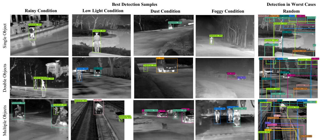
Fig. 14 Typical detection results of various atmospheric conditions in our created night time dataset. Column (1) shows detection results under rainy condition, column (2) shows detection results under low
