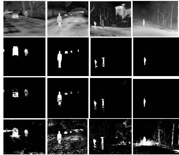
(a) Low Light (b) Dust (c) Rain (d) Fog Figure 3. Typical segmentation results for various atmospheric conditions in our created night time dataset. row (1) shows input frames, row (2) shows ground truth, row (3) shows ViBe results (best), row (4) shows CodeBook results (worst).
