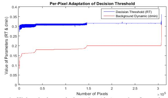
Fig. 6. Higher background dynamics ( $d_{\min}$ ) require faster threshold increments in the decision threshold ( $R_T$ ) and the thresholds gradually decrease for in low background dynamic values.
