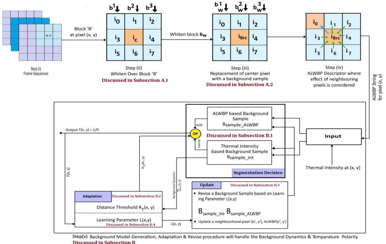
Fig. 3. Proposed system pipeline for background segmentation from thermal video sequences in adverse weather conditions.
